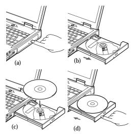
Figure 4-5 Loading/Ejecting a DVD/CD
